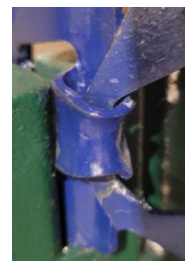
Figure 4: Suitable mark in the "GO" area
