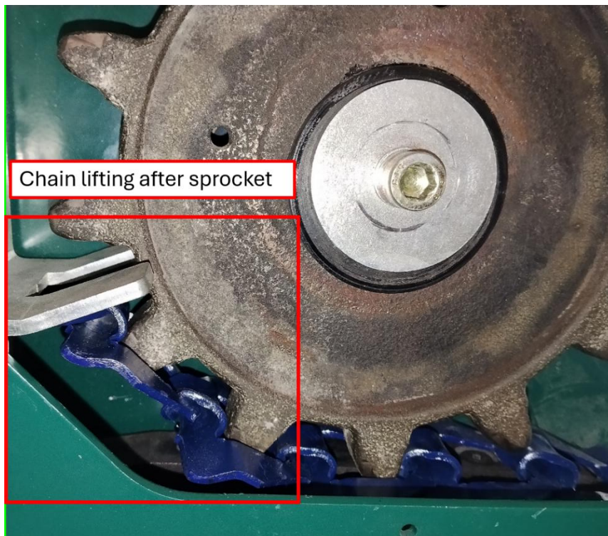
Figure 19: Lifting after sprocket - Under tension
